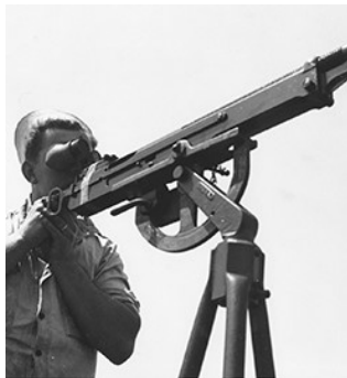
U.S. Navy sailor demonstrates use of the Polaroid Optical Ring Sight attached to anti-aircraft gun, ca. 1944 Polaroid Corporation Records.
